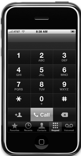
Figure 6-2. The Phone application is an example of a multiview application using a tab bar.
