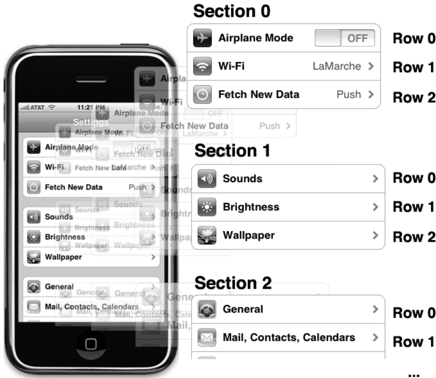
Figure 8-4. Sections and rows in a grouped table are obvious, but all tables support them.
