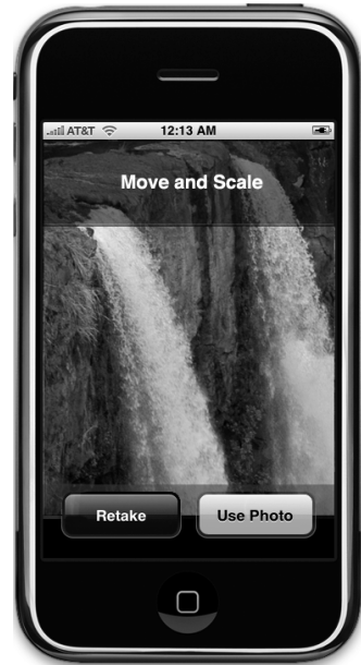
Figure 16-3. If you set allowsEditing to YES, the user will be able to zoom and crop images before returning to our application.
