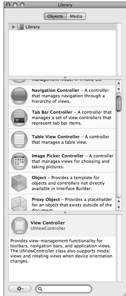
Figure 2-6. The Library palette, where you'll find stock objects from the UIKit that are available for use in Interface Builder
