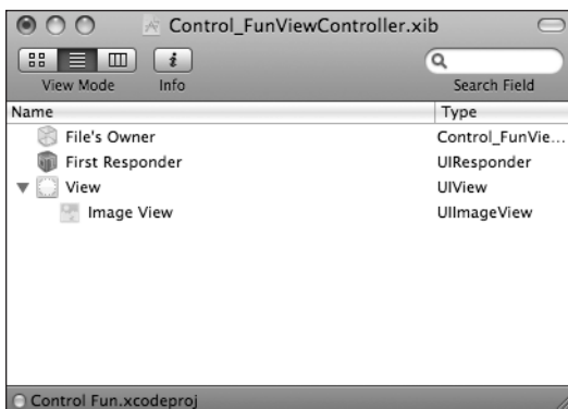
Figure 4-7. Putting the nib's main window in hierarchical view and drilling down to subviews
