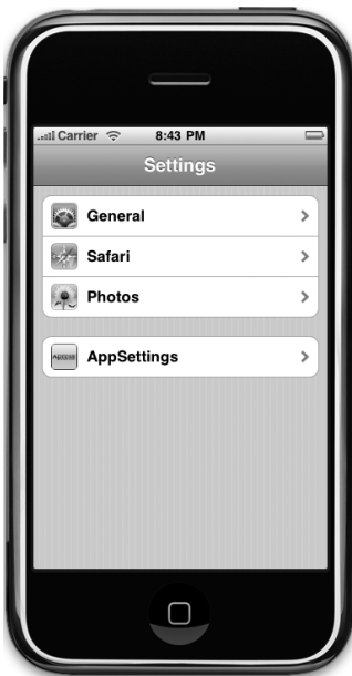
Figure 10-3. The settings application showing an entry for our application in the simulator
