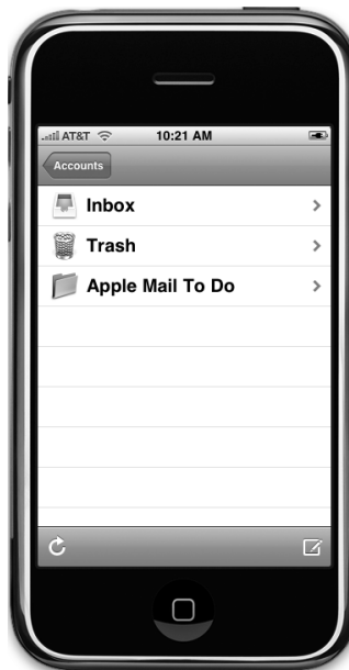
Figure 6-3. The iPhone Mail application is an example of a multiview application using a navigation bar.
