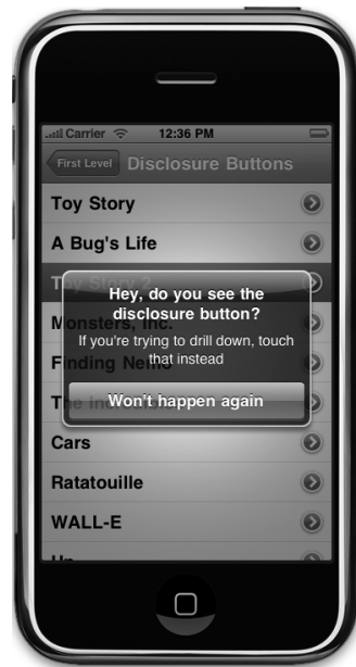
Figure 9-14. Selecting the row does not drill down when there is a detail disclosure button visible.
