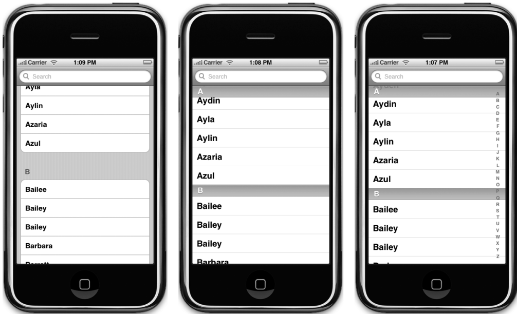
Figure 8-3. The same table view displayed as a grouped table (left); a plain table without an index, (middle); and an plain table with an index, also called an indexed table (right)
