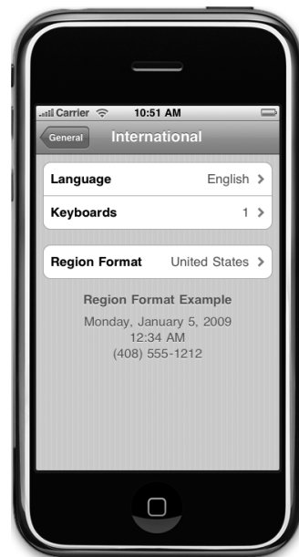
Figure 17-7. Changing the language and region, the two settings that affect the user's locale
