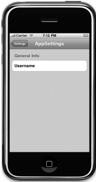
Figure 10-14. Our root view in the Settings application after adding a group and a text field
