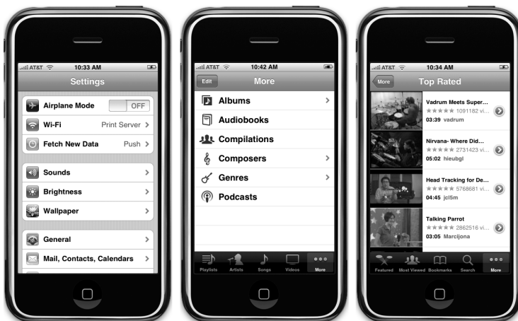
Figure 8-1. Though they all look different, the Settings, iPod, and YouTube applications all use table views to display data.
