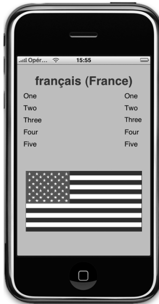
Figure 17-3. The nonlocalized application run on an iPhone set to use the French language
