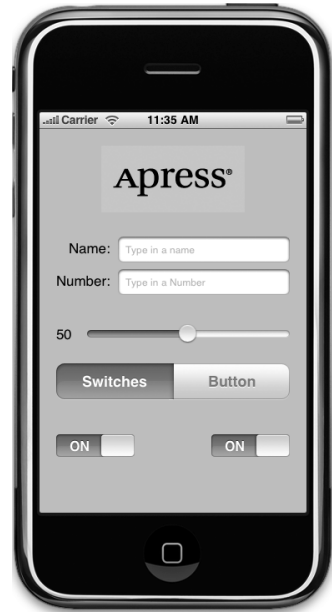
Figure 4-1. The Control Fun application, featuring text fields, labels, a slider, and several other stock iPhone controls
