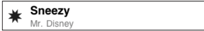
Figure 8-10. The subtitle style shows the detail text in smaller, gray letters below the text label.
