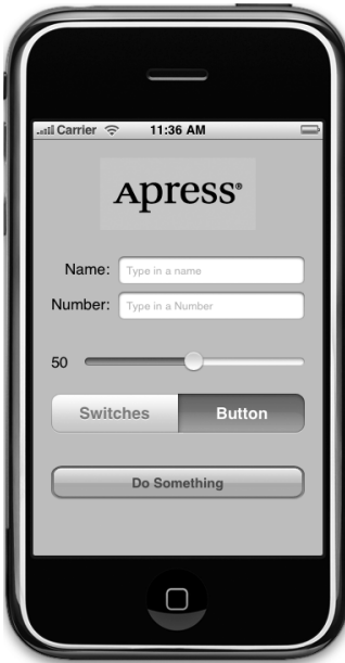
Figure 4-2. Tapping the segmented controller on the left side cause a pair of switches to be displayed. Tapping the right side causes a button to be displayed.
