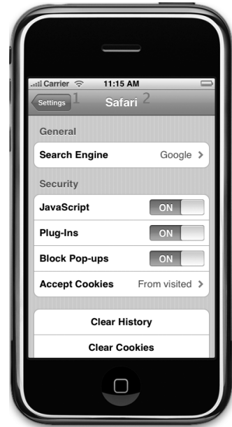
Figure 9-1. The Settings application uses a navigation controller. In the upper left (1) is the navigation button used to pop the current view controller off the stack, returning you to the previous level of the hierarchy. The title (2) of the current content view controller is also displayed.
