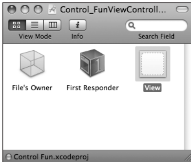
Figure 4-17. The nib's main window has three icons. The third one, labeled View , is our nib's content view.
