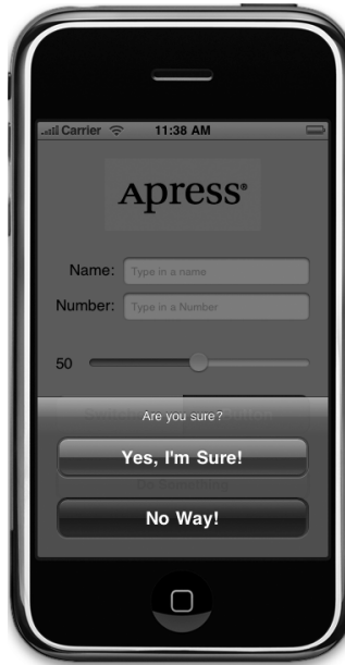
Figure 4-3. Our application uses an action sheet to solicit a response from the user.
