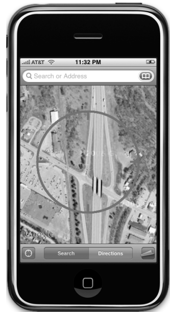
Figure 14-1. The Maps application uses Core Location to determine your current location. The blue circle is a visual representation of the horizontal accuracy.
